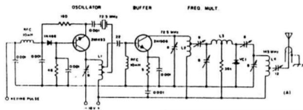
OSCAR 1 Beacon Transmitter: 140 mW at 145 MHz.
