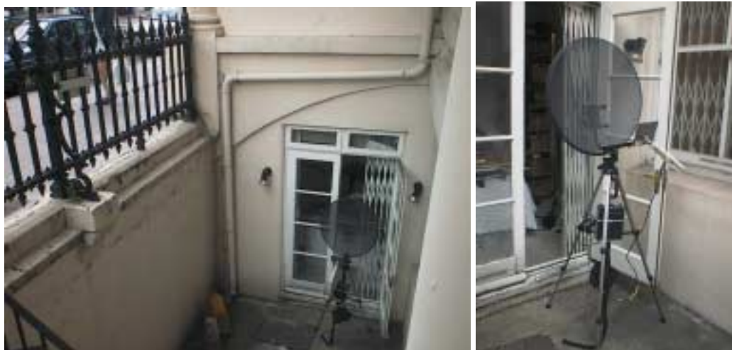
AO-40 reception at 8' below ground level
